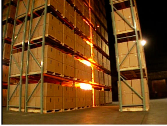
Figure 11: A large-scale fire test as the flame spreads up through the flue space between the packed commodity boxes [46].
